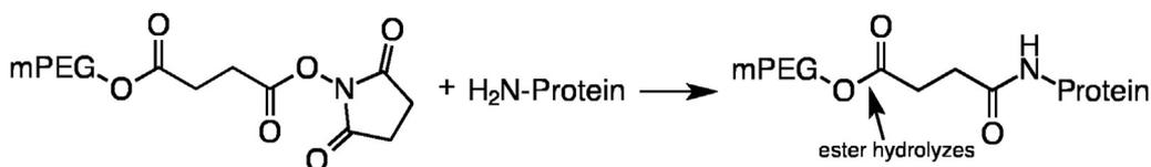
**Figure 11.** Conjugation of PEG to a protein by a SS linker. Ester hydrolysis may result in removal of PEG at the position indicated by the arrow.
