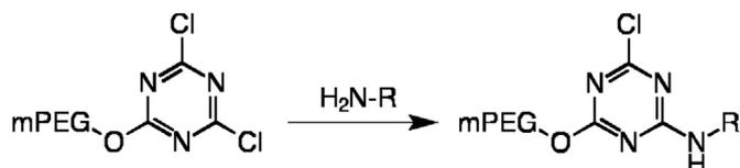
Figure 3. PEGylation of primary amines in proteins (H<sub>2</sub>N-R) by PEG dichlorotriazine.
