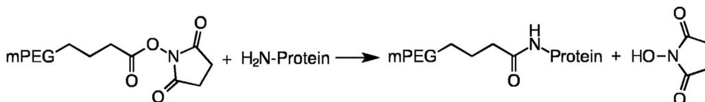
**Figure 16.** PEGylation reaction used for synthesis of Mircera® with an mPEG succinimidyl butanoate reagent attaching primarily lysine 52 and 56.
