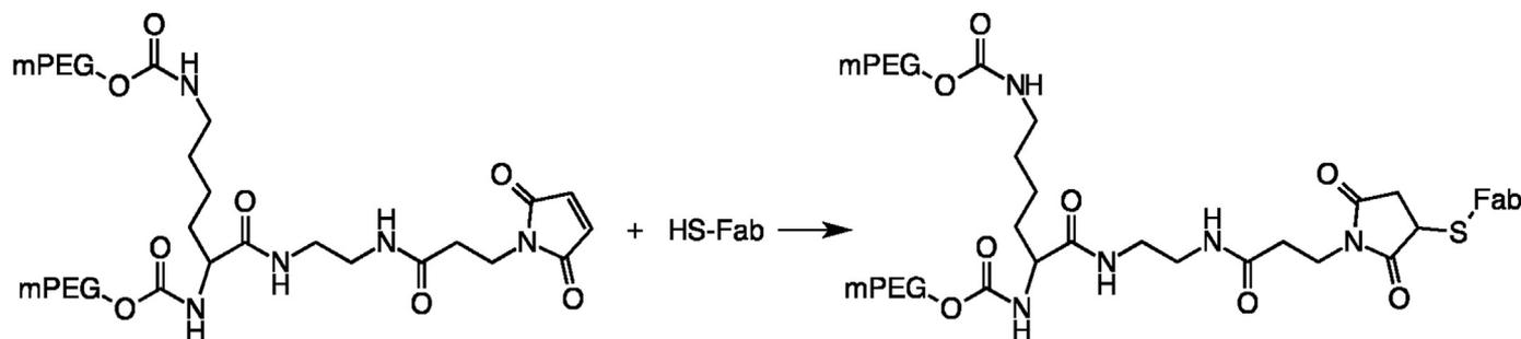
Figure 23. Synthesis and structure of Cimzia® a thiol-engineered PEGylated antibody fragment conjugate.
