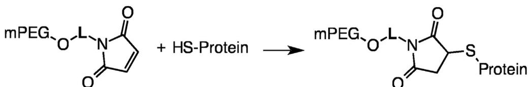
**Figure 22.** PEGylation reaction used for selective thiol PEGylation with a PEG maleimide reagent (L: linker group between the PEG and active head group).
